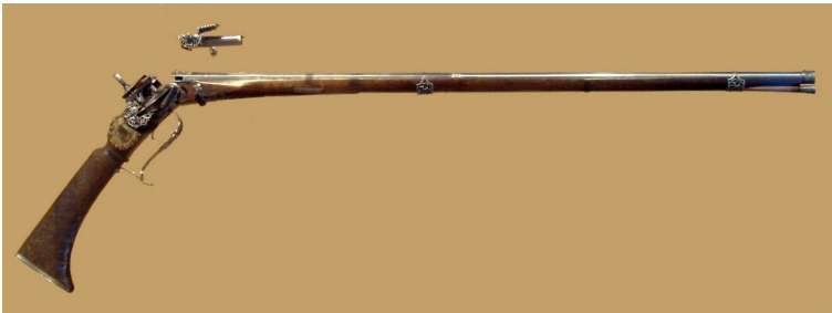
Figure 5.10 Early breech loader w/ fitted cartridge
