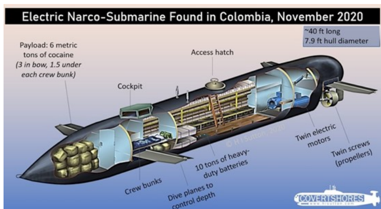
Figure 2.11 Electric Narco-Submarine (Sutton, 2020)
