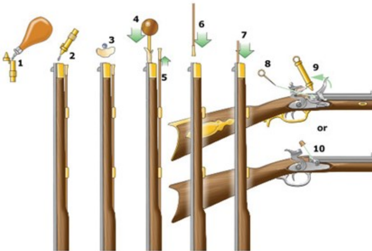
Figure 5.6 Loading Steps of a Muzzle loader
