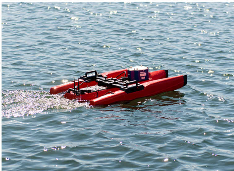
Figure 4.10 Q-Boat 1250 designed specifically for shallow water applications
