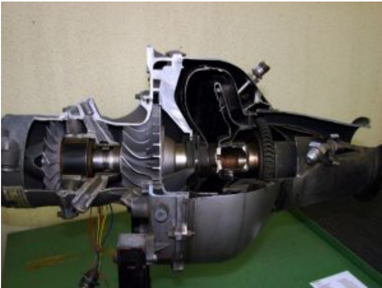
Figure 1.2 Cross section of a typical gas turbine engine. Courtesy of Tilyudai and reused under license CC BY-NC-SA 2.0. To view a copy of this license, visit https://creativecommons.org/licenses/by-nc-sa/2.0/ .
