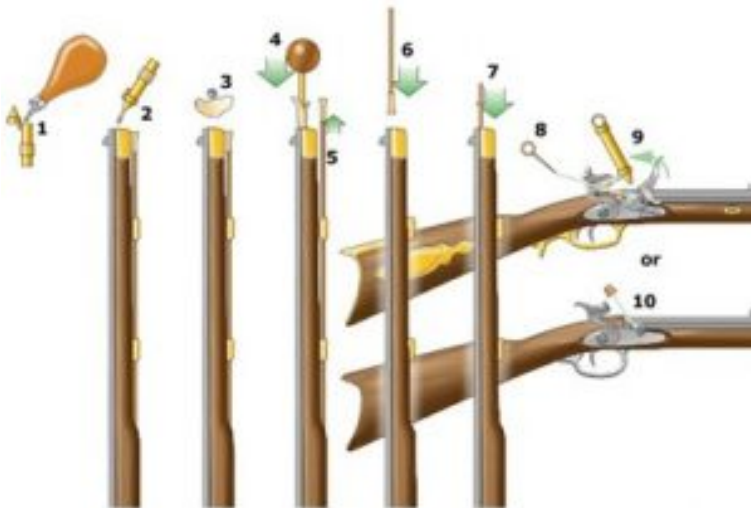
Figure 5.6 Loading Steps of a Muzzle loader
