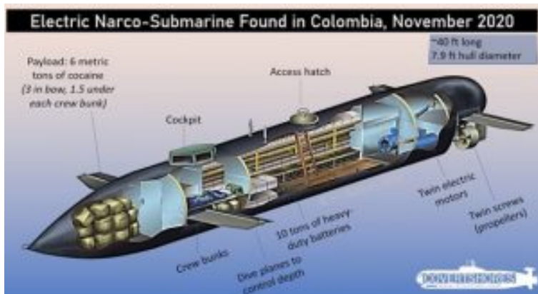
Figure 2.11 Electric Narco-Submarine (Sutton, 2020)
