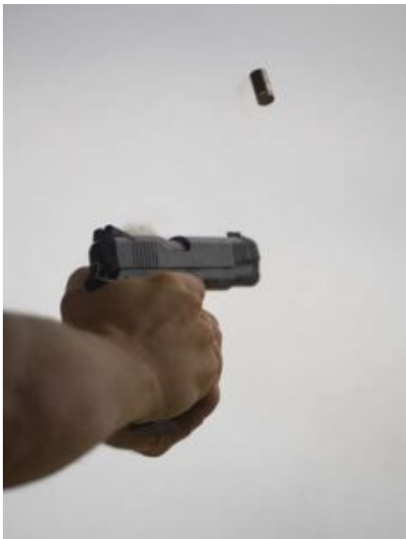
Figure 5.17 Shell ejection and reloading using excess gas
