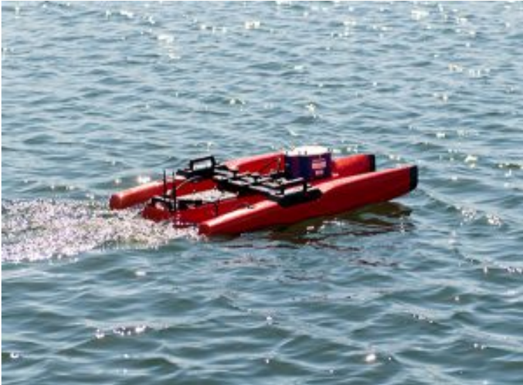
Figure 4.10 Q-Boat 1250 designed specifically for shallow water applications
