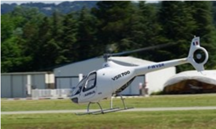
Figure 2.12 VSR 700 OPV (VSR700 demonstrator performs first autonomous flights, 2017)
