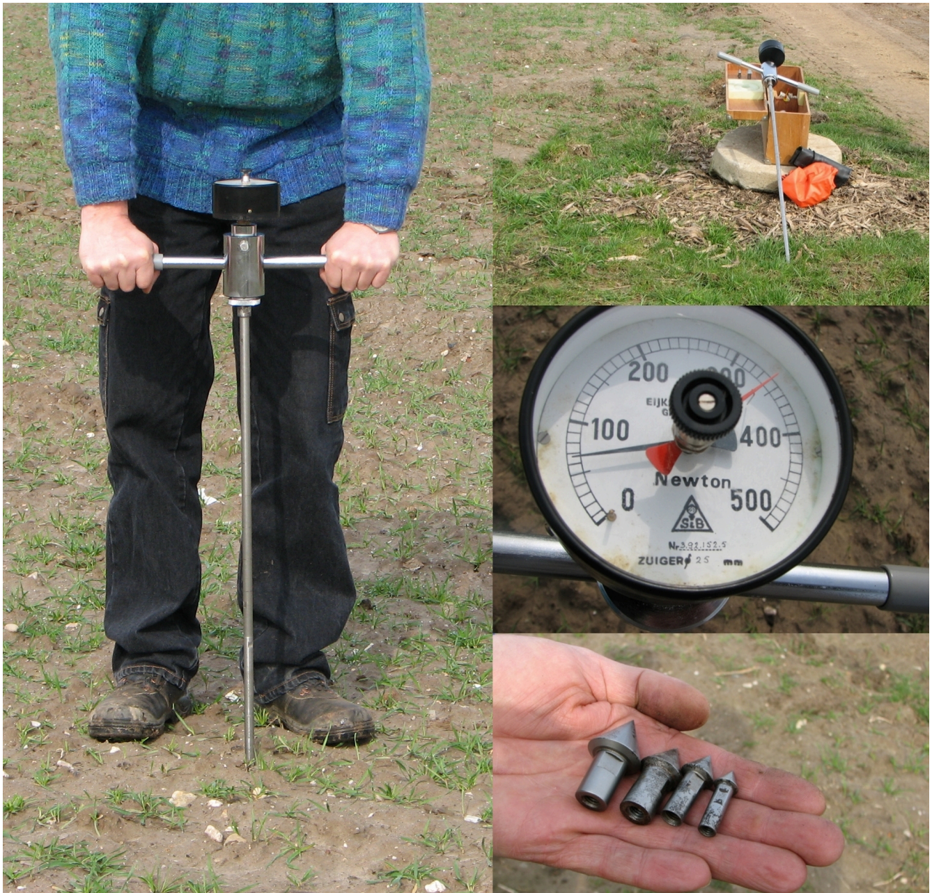
Figure 6.1. A handheld penetrometer being used in the field (left), associated equipment (top right), power meter (center right), and cones (bottom right). Photograph courtesy of HPsy.
