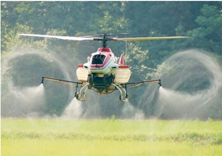
Figure 2.5 Agriculture Drone is spraying pesticides on crops.
