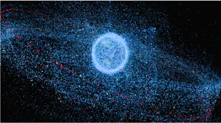
Figure 14.5. Computer simulation of tracked objects in Earth's orbit. Red, yellow, and green objects are representations of active satellites and debris in the GEO and MEO.
