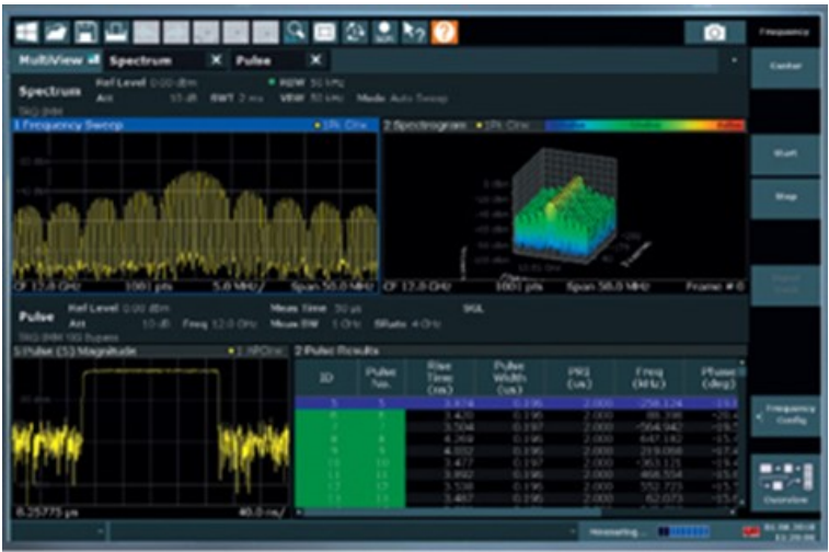
Figure 11.10: Analyzing a Radar Pulse Using an R&S Spectrum Analyzer
