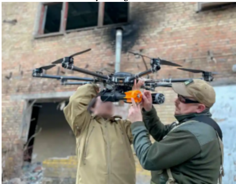
Figure 1.10 Field assembly of a drone capable of thermal imaging and delivery of 1.5kg bombs
