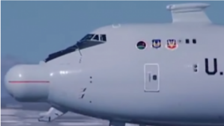
Figure 10.7: LASER platform mounted on Boeing 747
