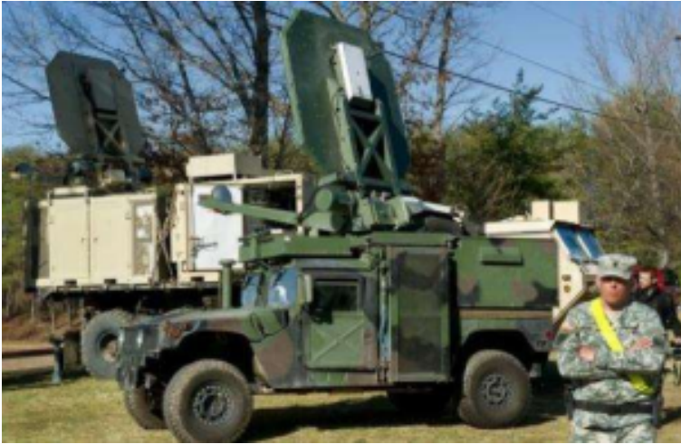
Figure 11.6A Two styles of US Marine Corps trucks are seen carrying the Active Denial System, March 9th, 2012, at the US Marine Corps Base Quantico, Virginia. The non-lethal weapon projects a strong electromagnetic beam up to 1000-meters
