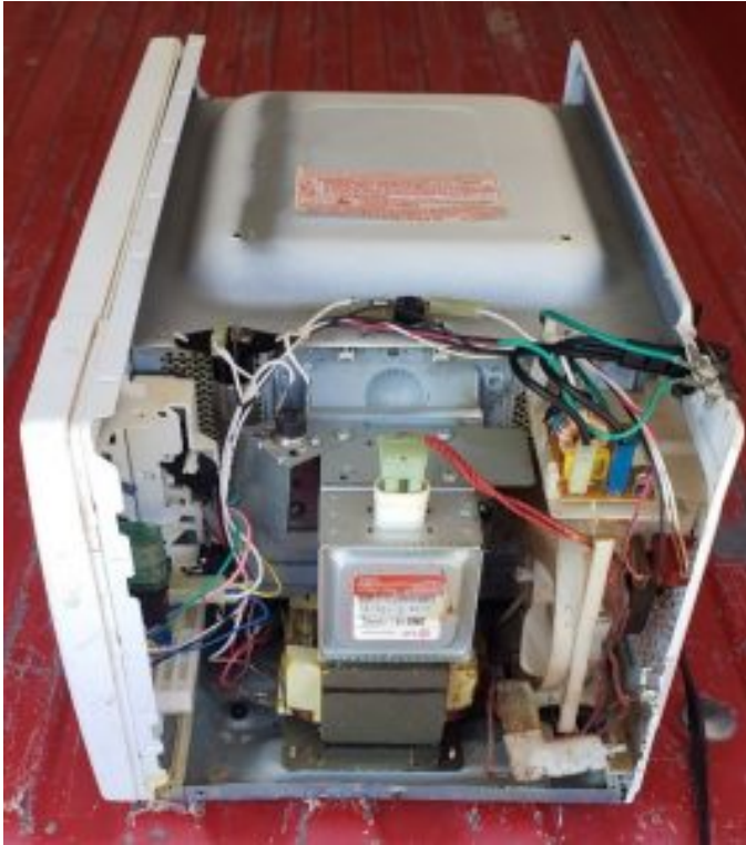
Figure 11.3: Inside of ordinary kitchen microwave oven
